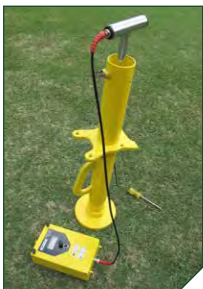
▲ Clegg hammer measures the surface hardness of the pitch.
